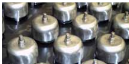
► Figure 2. Bubble cap trays require a large amount of metal.
