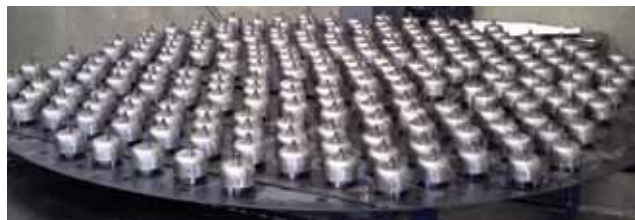
► Figure 2. Bubble cap trays require a large amount of metal.
