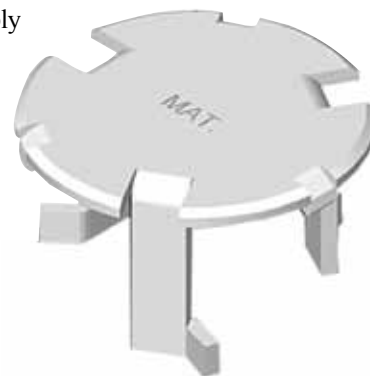
► Figure 3. Round valves require less material than bubble caps.
